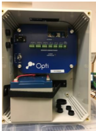
Fig. 1: Opti Monitoring Panel with battery installed (left), Opti Monitoring Panel pole mount kit (right)
