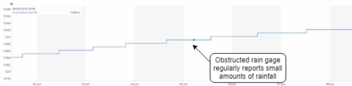
**Figure 10:** Rain gauge obstruction readings
