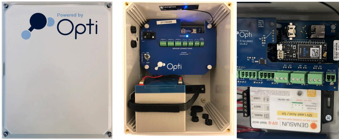
**Figure 2:** Opti Monitoring Panel cover, interior, and the OptiThunder cellular gateway and Genasun Charge Controller (left to right).
