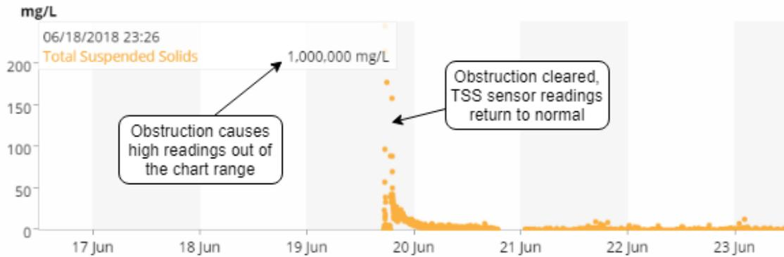
**Figure 11:** TSS sensor obstruction readings
