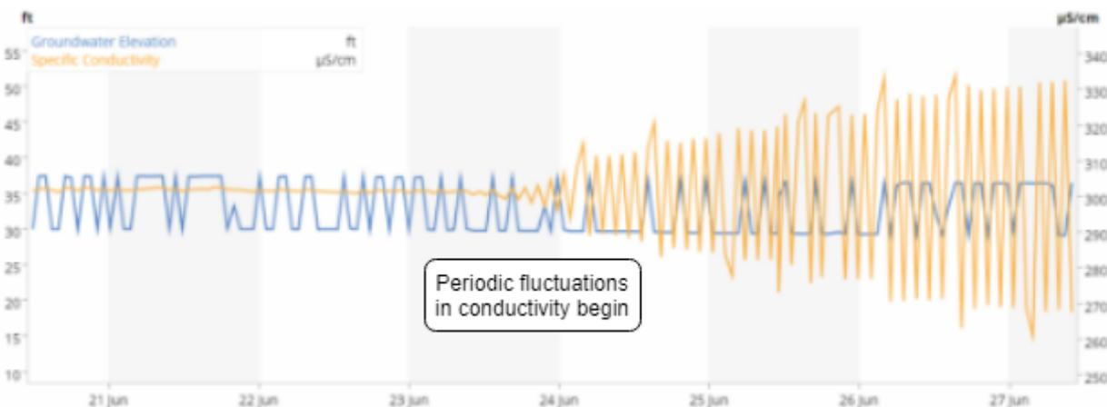
**Figure 6:** Biofouled conductivity readings
