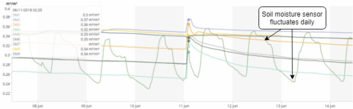
**Figure 7:** Periodic soil moisture sensor readings
