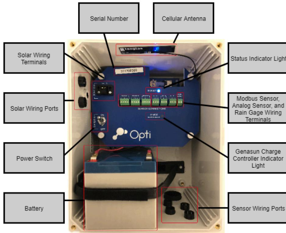
**Figure 3:** Opti Monitoring Panel annotated with major components
