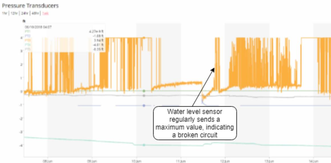
**Figure 5:** Faulty water level sensor readings
