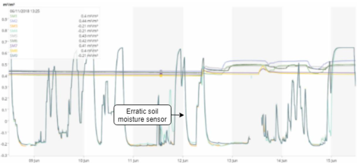
**Figure 8:** Soil moisture sensor failure readings
