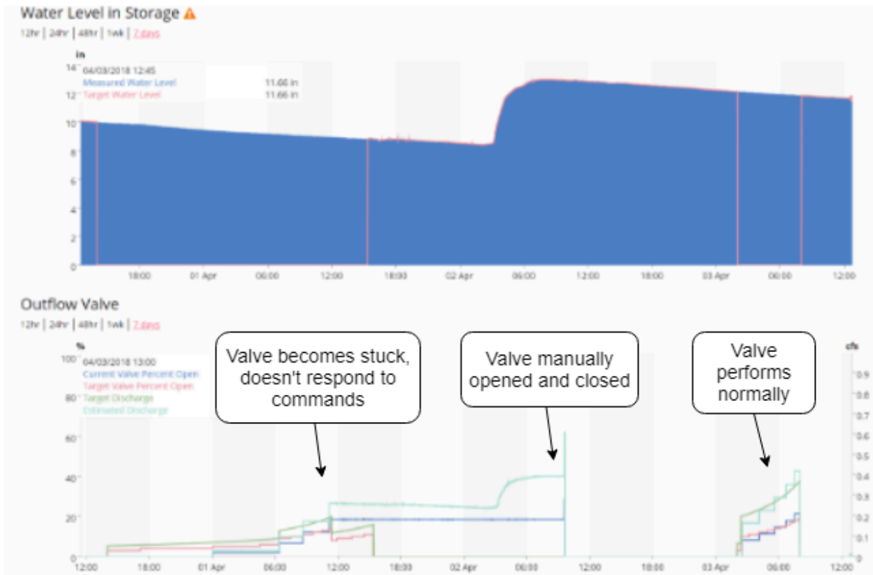
Figure 8: Opti dashboard during a valve clog
