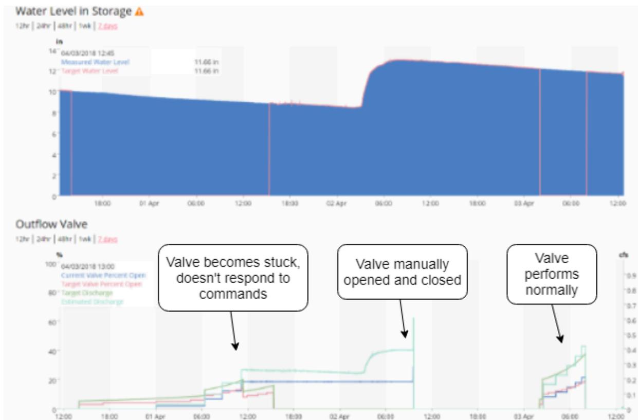
**Figure 7:** Opti dashboard during a valve clog
